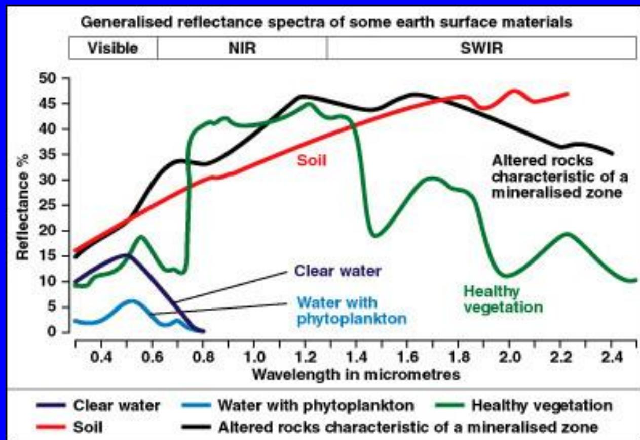
The electromagnetic radiation is reflected by the surfaces depending on their physical and chemical characteristics.
