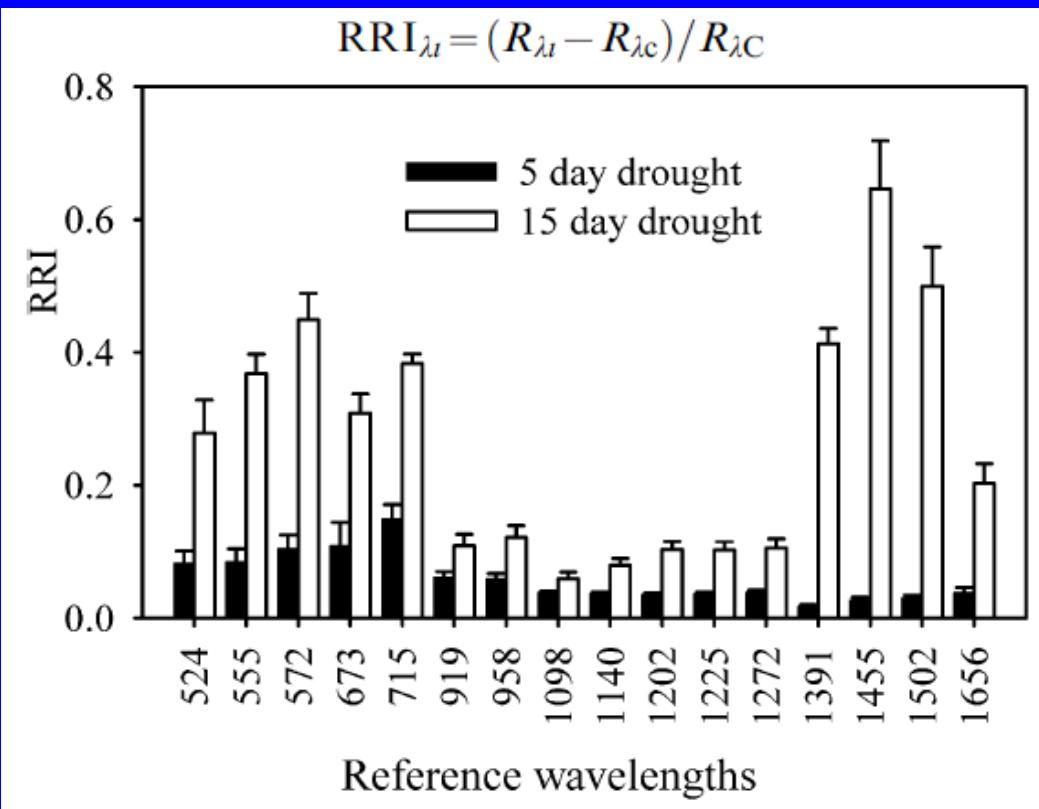
Relative reflectance increment (RRI) determined at different reference wavelengths in water-stressed olive saplings after five and 15 days from the onset of water stress.
