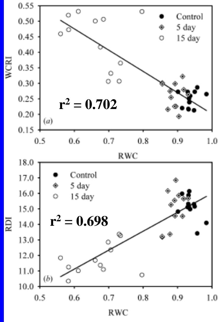
Relationships between relative water content (RWC) and (a) water content reflectance index (WCRI) and (b) relative depth index (RDI).
