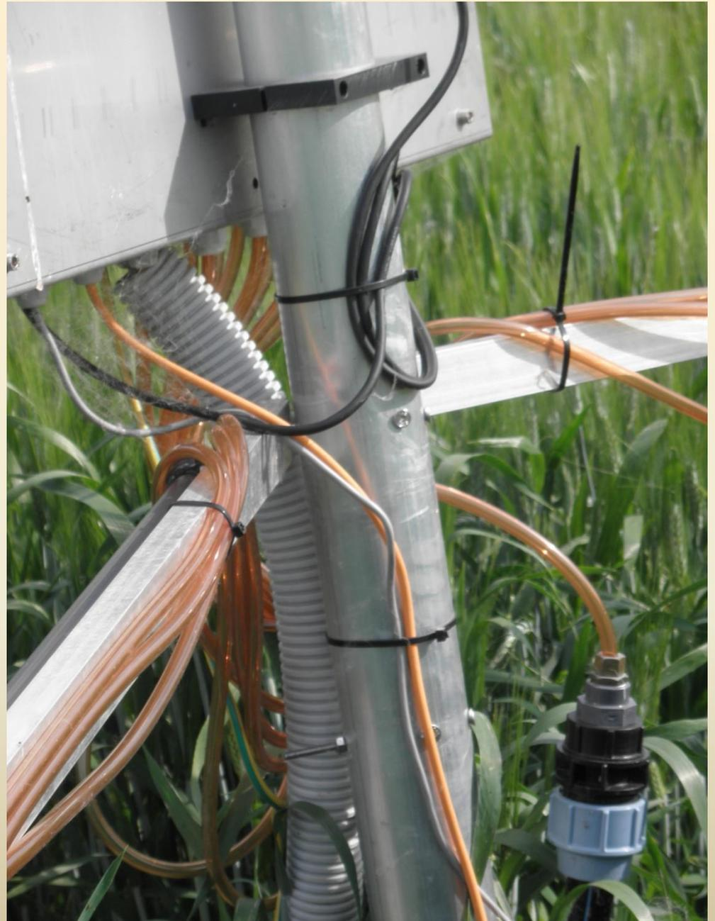
**The CO<sub>2</sub> reading is obtained using an infrared open path gas analyzer Vaisala model Carbocap.**
