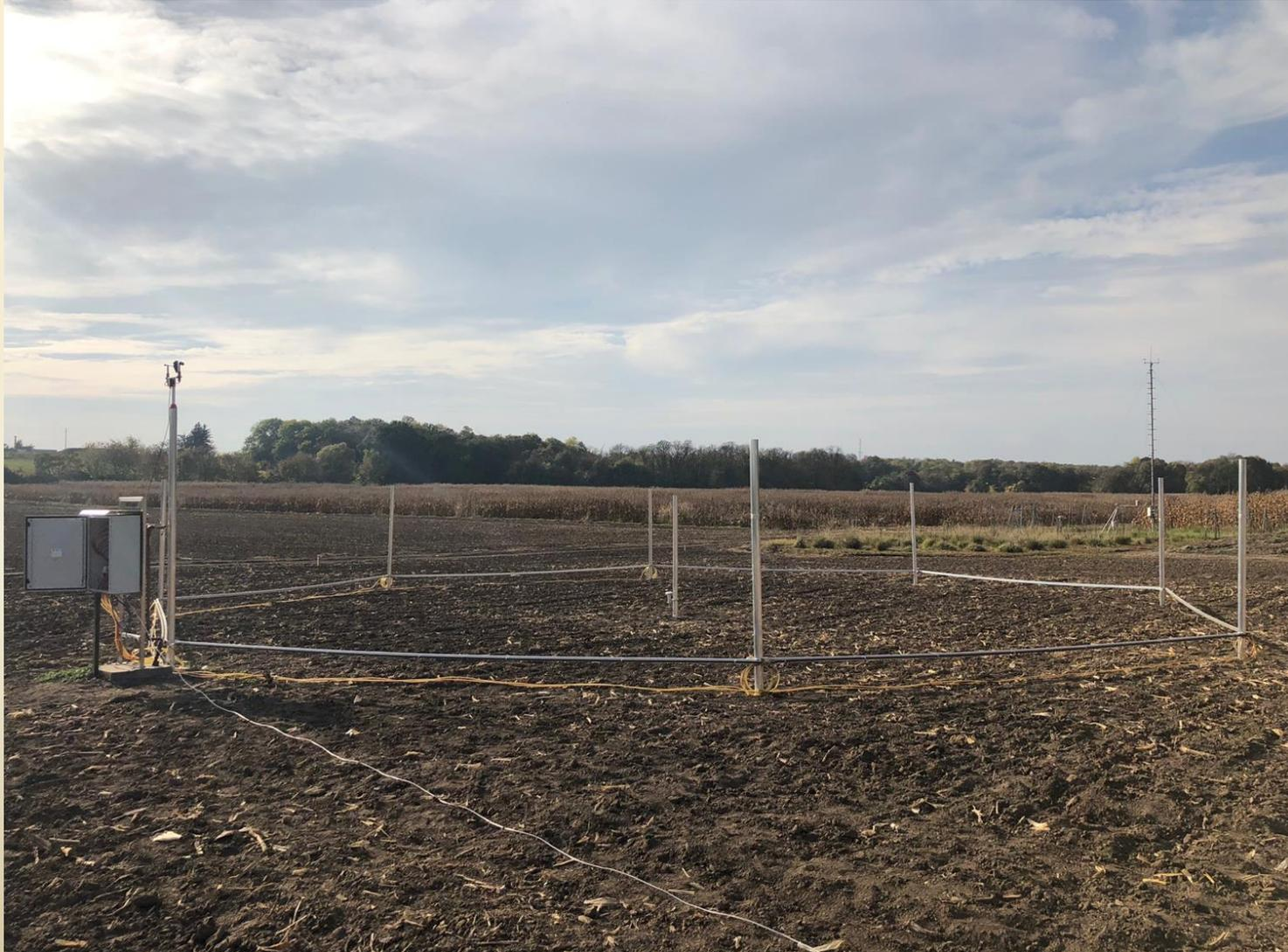
**Each ring is constituted by a control unit and a series of 8 laser drilled pipes to release CO2. The release system is made by one storage tank holding the supply of liquid CO2 at -180° C, radiators bringing the gas to ambient temperature and a vaporizer that ensures non-interrupted supply of CO2 to the rings through underground pipes.**
