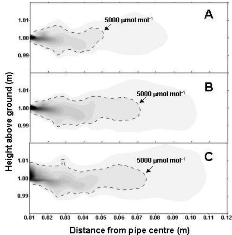
Furthermore, the microscopic holes (0.2mm diameter) laser-drilled into the outer circumference of these pipes, allow CO<sub>2</sub> to be ejected out at sonic speed against the incoming air mass to maximise mixing of CO<sub>2</sub> with ambient air.
