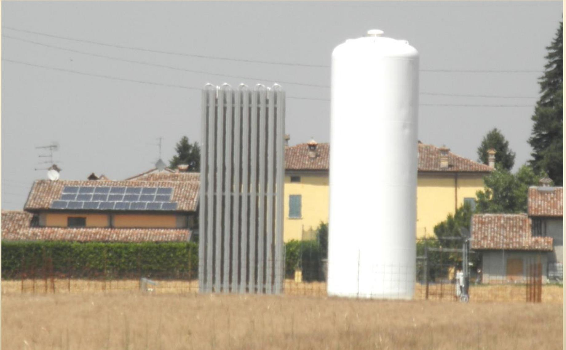
**The release of CO<sub>2</sub> is controlled through a system of valves connected to the 8 laser drilled pipes forming the sides of the ring itself. The pipes are installed on adjustable supports, which allow to raise the ring during the vegetation growth.**
